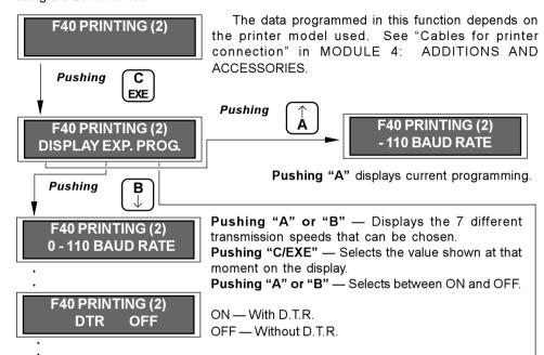
Some printers cannot print at the same speed at which the payout unit transmits data. If the printer does not have memory for storing the data transmitted by the payout unit, the D.T.R. command can be used.
