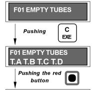
When the F01 submenu is accessed, four possibilities appear, TB\_A/TB\_B/TB\_C/TB\_D, which can be accessed with A, B, C, or D, respectively.
