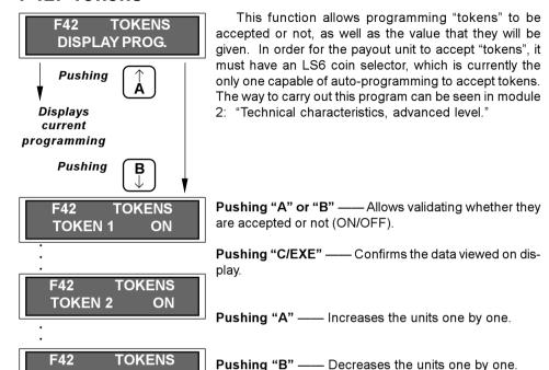
Pushing "C" —— Allows programming the next digit.
