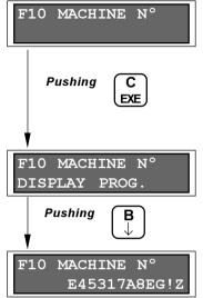
It allows personalising the payout unit (and therefore the machine where it is installed) with a set of twelve characters (numbers, letters, or symbols).
