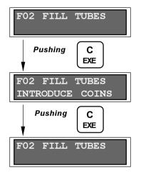
This function allows coins to be introduced into the returner tubes for later use as change.
