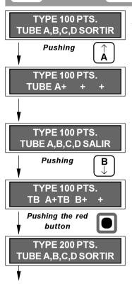
In order for one coin to go to two tubes at the same time, for example the 100-peseta coin to go to tubes A and B. follow the procedure indicated on the left...
