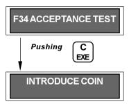
This allows performing quick verification of coins that are legal tender and that are possible frauds, verifying if the selector accepts the introduced coin as good or if it is rejected.
