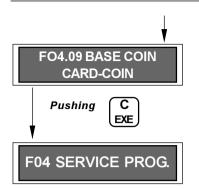
Azkoyen payout units are prepared to be connected to a "pre-paid card reader." This function allows selecting whether the payout unit as well as the card reader will operate with the base coin programmed in the payout unit (see function F32) or with what is programmed on the pre-paid card (1 peseta).
