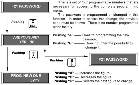
Once this function has been entered, it cannot be exited without programming a number. Even though four zeros are programmed, this will be the secret number. The only way to erase it is to erase the RAM (see F22), and in order to do that the password must be known.
