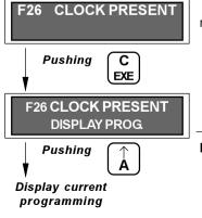
If ON is programmed in this function, the payout unit reflects the time on the machine LED display.
