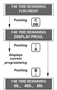
When the payout unit cannot provide change after a service because its returner tubes are out of change, the time that the payout unit will keep as credit on display the amount that should be returned as change can be programmed.
