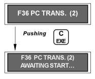
The payout unit will start transmitting after receiving a "T" character that is sent from the computer. When the transmission has been completed, the payout unit will wait for a series of responses from the computer:
