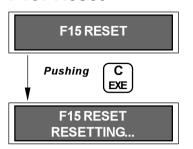
This is used to void a possible breakdown from the payout unit memory after having eliminated or corrected the problem that caused it.
