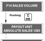
This allows viewing the accounting for completed sales since the last time it was zeroed out.
