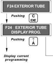
It is possible to attach a manually loaded exterior tube to the payout unit that would act as support for the base coin that is used for change. If there are 5-, 25-, and 100-peseta coins, the exterior one would return 5-peseta coins.
