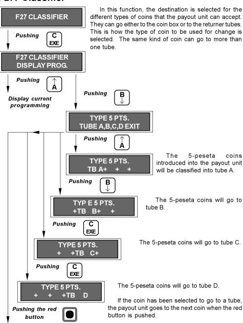
TYPE 5 PTS. COIN BIN If the coin has not been selected to go to any tube, then it will be sent to the coin bin and the next coin is taken.
