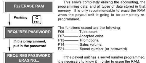
If the RAM is erased, it will be necessary to remove the change coins (if there were any) and to introduce them again since the count in function F06 has returned to zero.
