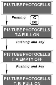
This allows verifying the proper operation of the tube level detectors (the optical sensors), as well as their possible wear or the accumulation of dirt.
