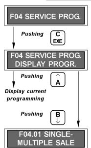
**Pushing "A"** —— Single sale. After carrying out the sale, the payout unit provides the corresponding change. **Pushing "B"** —— Multiple sale. The payout unit keeps the change on display as credit. It gives this change when the machine coin return button is pushed.
