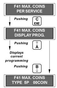
This function allows programming the maximum number of each type of coin that the payout unit is going to accept for carrying out a sale. This value can be programmed between 00 and 99.
