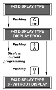
This function allows choosing the external display type connected to the payout unit:
