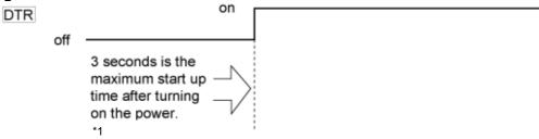
\*1:HOST should be transmitted data after DTR Signal turns ON.
