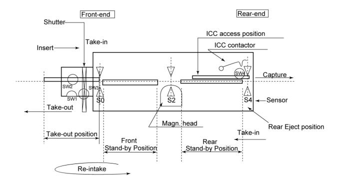
S0: Front end sensorS2: Mid-position sensorS4: Rear-end sensor
