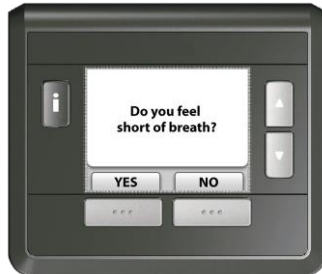
Figure 6. The RTX337x has 5 buttons on the front. Two selection (soft) buttons below the display, scroll up, scroll down on the right of the display and an info button on the left of the display. Two buttons for volume up and down can be found on the side.
