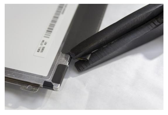
Figure 23. Cutting the corner of the logic board
