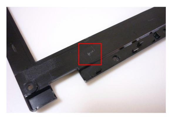
Figure 18. Right inner LCD bezel clip is removed (the left one looks similar)
