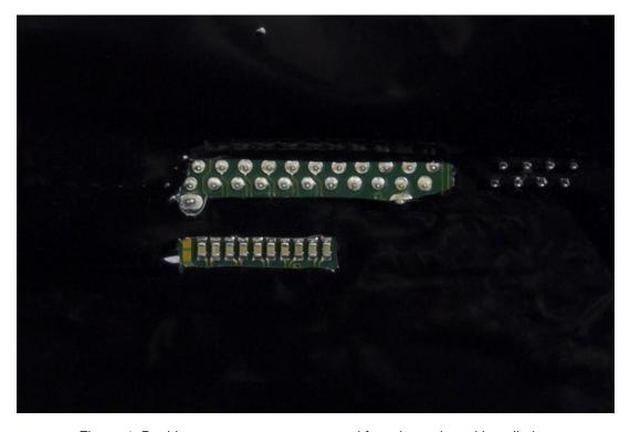
Figure 4. Docking connector area prepared for adapter board installation
