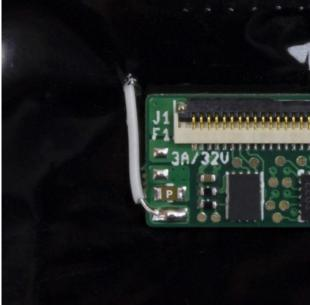
Figure 15. Auxiliary power wire pad on the adapter board
